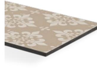
Compact high pressure laminate of standard quality with individual digital printed motifs based on EN 438-4:CGS. With uniform black-coloured core and white reverse. Our well-known Individual world from just 1 piece upwards, where your image files can be used as a motif.
