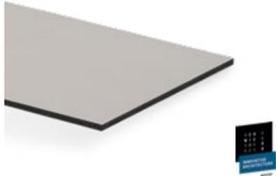
Compact high pressure laminate for outdoor use in flame-retardant quality according to EN 438-6:EDF / intensive decors according to EN 438-6:EGF. With uniform black-coloured core and single-sided decorative acrylic lacquer on the top side and decorative melamine resin surface on the reverse.
