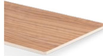
Fire protection panel with IMO classification "Low Flame-Spread Surface Material" of primarily mineral constituents with uniform white-coloured core and decorative melamine resin surface on both sides.
